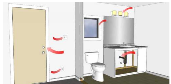
Above-grade wall air sealing locations.
