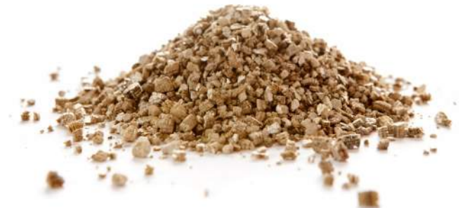
Vermiculite attic insulation potentially containing asbestos fibres.
