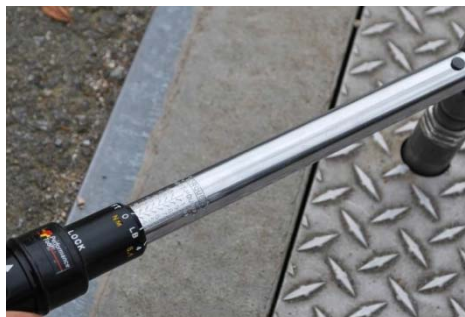
Figure 3 – Puzzle bolt tightened by torque wrench
