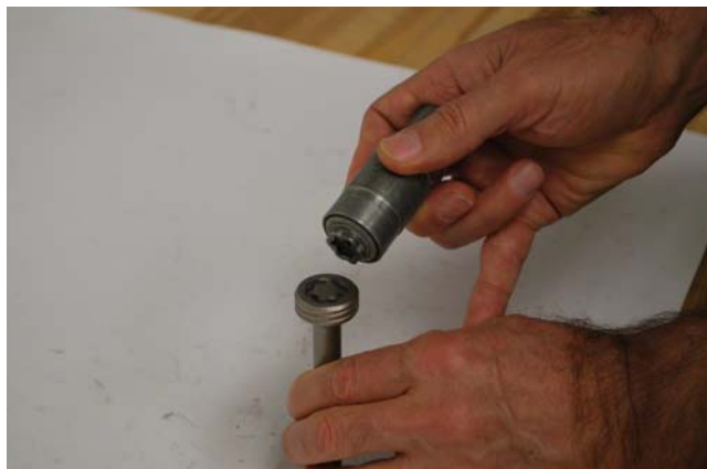
Figure 1 – Puzzle bolt unique driving pattern and outer thread with socket shroud pulled back for alignment of two matching patterns
