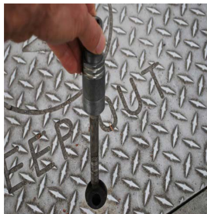
Figure 2 – Puzzle bolt engaged
